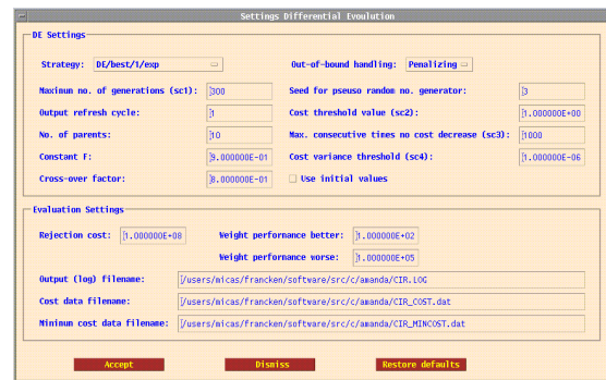
Fig. 6. The differential evolution algorithm and cost function evaluation settings.
