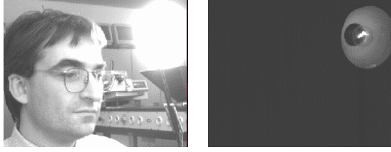
Figure 4: Two images captured from a high dynamic range lab scene with light bright bulb representing the longest (left) and shortest (right) integration time.
