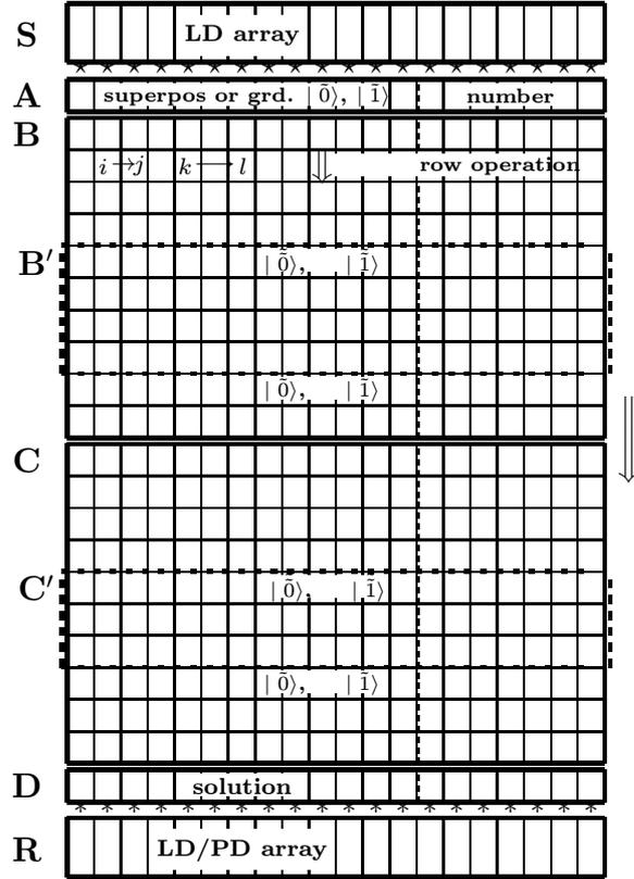
Figure 2: A solid state quantum computer; (S) light sources, (A) input port, (B) first computing field, (C) second computing field, (D) output port, and (R) probing and detecting elements.
