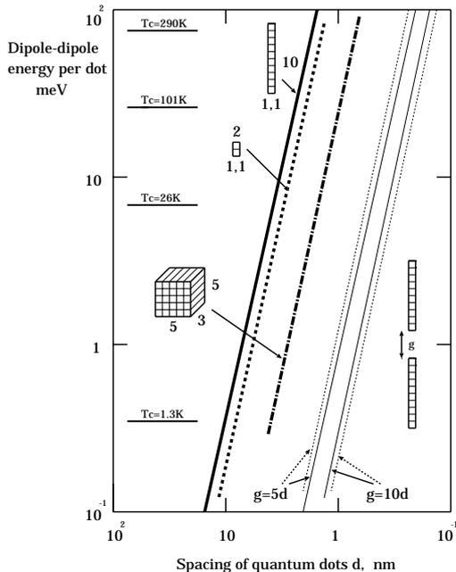
Figure 1: Dipole-dipole interaction energy per quantum dot as the function of the spacing ( $d$ ) of quantum dots, and with inter-block separation ( $g$ ) as the parameter.
