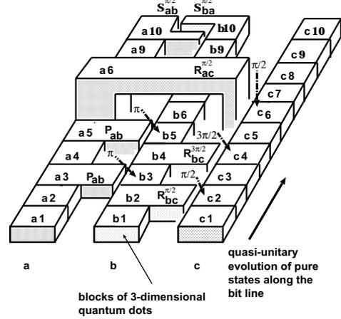
Figure 3: A solid block CCN gate, combining two CN gates ( $P_{ab}$ ), two  $\frac{\pi}{2}$  controlled rotators ( $R_{bc}^{\pi/2}$  and  $R_{ac}^{\pi/2}$ ), one  $\frac{3\pi}{2}$  controlled rotator ( $R_{bc}^{3\pi/2}$ ), and a pair of  $\frac{\pi}{2}$  controlled phase shifters ( $S_{ab}^{\pi/2}$  and  $S_{ba}^{\pi/2}$ ). Arrows with  $\pi$ ,  $\frac{\pi}{2}$ , and  $\frac{3\pi}{2}$  denote the respective photonic pulses.
