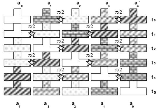
Figure 5: Conceptual scheme of a bit reversal permutation circuit with an odd number of bits, consisting of the qubit swap ( $\Pi_4$ ) gates activated by negative electromagnetic  $\frac{\pi}{2}$  pulses;  $|a_0\ a_1\ a_2\ a_3\ a_4\rangle \rightarrow |a_4\ a_3\ a_2\ a_1\ a_0\rangle$ .
