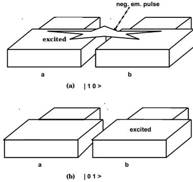
Figure 4: A qubit swap ( $\Pi_4$ ) gate activated by a negative electromagnetic  $\frac{\pi}{2}$  pulse. (a) before the pulse, bit a is excited representing  $|10\rangle$ , (b) after the pulse, bit b is excited representing  $|01\rangle$ .
