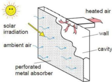
Figure 3 Example of an unglazed thermal solar wall
