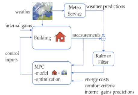
Figure 4 Example of an MPC formulation
