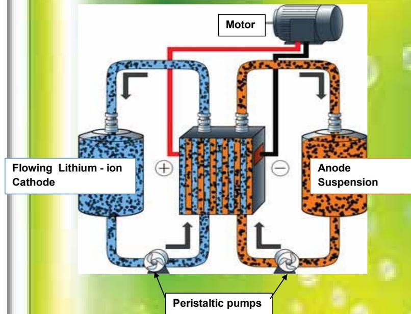
Figure 01. Schematic diagram of SSFC<sup>1</sup>
