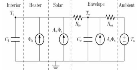
Fig. 2 Example RC-network thermal building model
