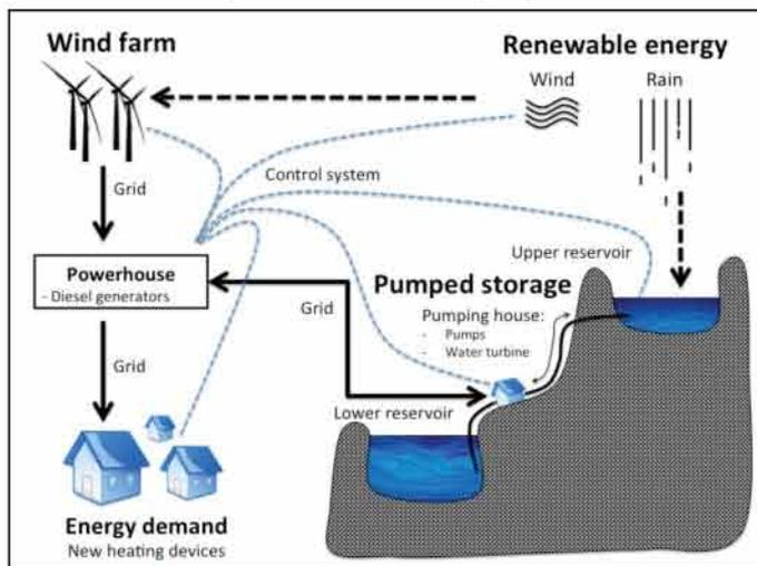
Schematic drawing of the supply system
