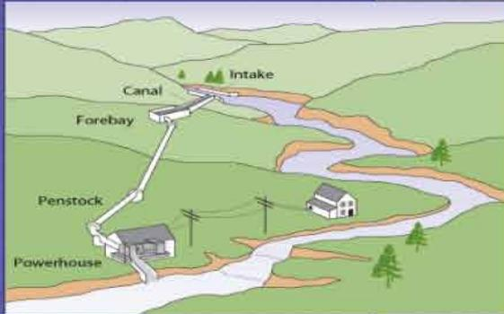
Figure 1. Schematic of a micro hydro power plant (photo: [www.mhpa.com](http://www.mhpa.com))
