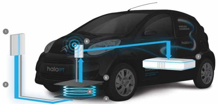
Image 1: The haloIPT wireless charging system. 1 – Power supply. 2 – Electrical wires. 3 – Transmitter pad. 4 – Wireless electricity transfer. 5 – Receiver pad. 6 – Data receiver. 7 – Battery <sup>7</sup>.
