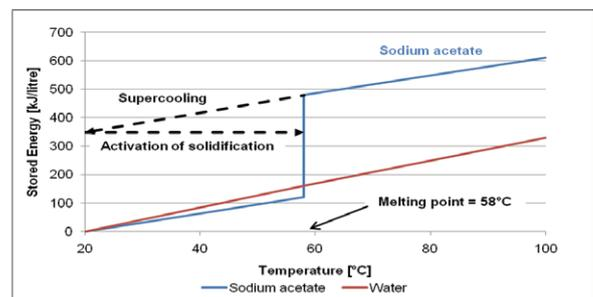
Fig. 1: Energy density of sodium acetate in the super cooling process compared to water.
