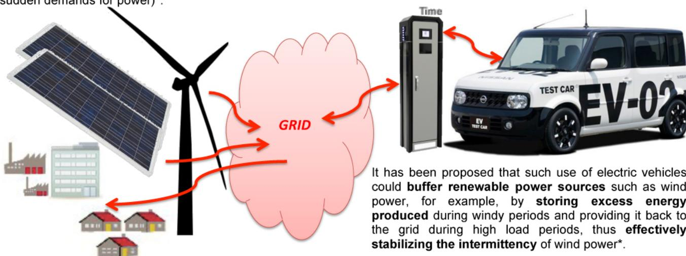
It has been proposed that such use of electric vehicles could **buffer renewable power sources** such as wind power, for example, by **storing excess energy produced** during windy periods and providing it back to the grid during high load periods, thus **effectively stabilizing the intermittency** of wind power\*.
