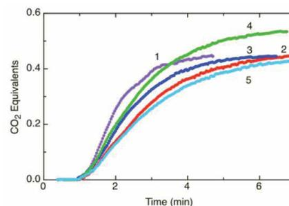
Fig 3. Lifetime/repeated CO<sub>2</sub> release from DBU and 1-Hexanol at 90 °C. Heating begins at 1 minute. [2]
