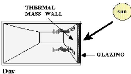
Figure 5 Glazed solar thermal wall
