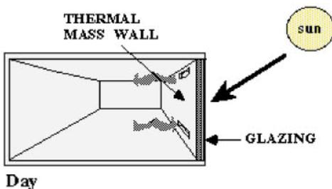
Figure 5 Glazed solar thermal wall
