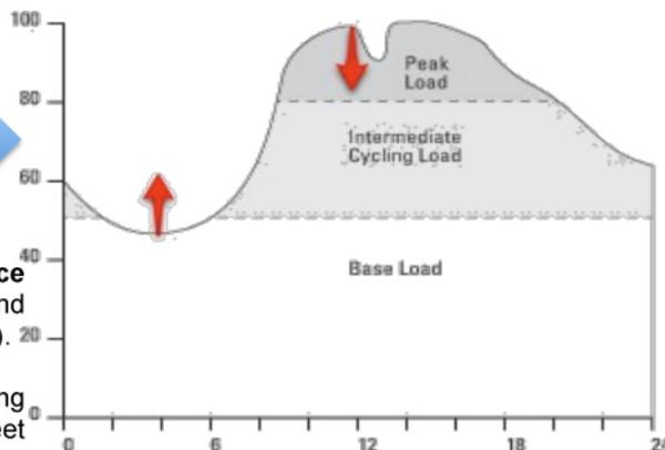
The concept allows **electric vehicles** to provide power to help **balance loads** by "valley filling" (charging at night when demand is low) and "peak shaving" (sending power back to the grid when demand is high).
