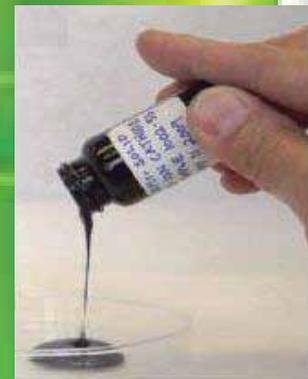
Figure 02. Semi-Solid Suspension containing  $\text{LiCoO}_2$ <sup>1</sup>
