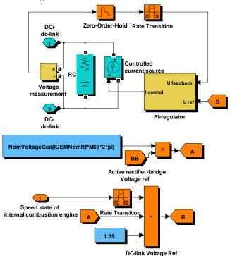
Fig. 6. The simulation model of the active rectifier
