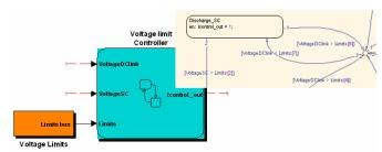
Fig. 4. The voltage control limits build on top of the current control loop with the Stateflow block.
