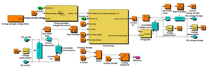
Fig. 3. The simulation model of the current controlled dc/dc converter
