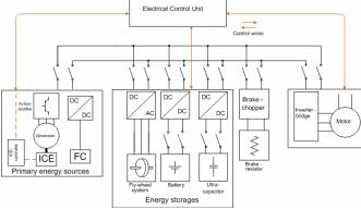
Fig 1. The layout of the series-hybrid drive train
