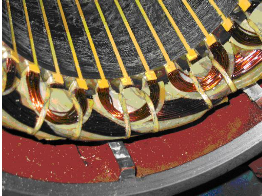
Figure 3.10 Auxiliary winding mounted into the stator slots
