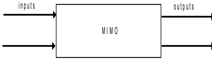
Figure 6 Schematic diagram of an MIMO system. In the MIMO-model, there may be many inputs and many outputs. In this representation, the transfer function is a matrix.
