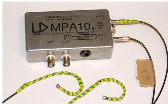
Figure 4.5: Sennheiser KE 4-211-2 microphones connected to UD-MPA10e preamplifier.
