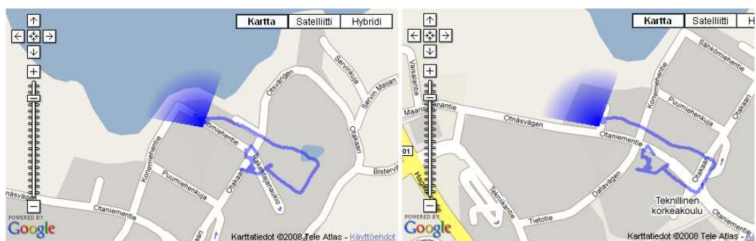
Figure 6.2: The offset error when directly plotting the positions on Google Maps visualised on the left. Corrected version on the right.
