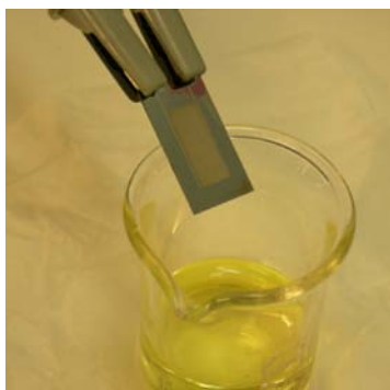
Figure 5.24 Small sized SC- \mu DGFC without the PDMS cover is being tested.
