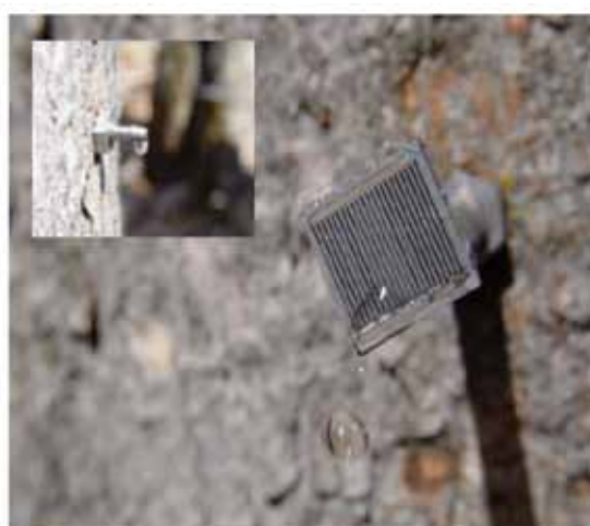
Figure 3.15 A simple sap harvesting device is inserted into a sugar maple tree. The sap dripping from the device is clearly visible. The device is meant to supply fuel to a \mu DGFC. Reproduced from [71].
