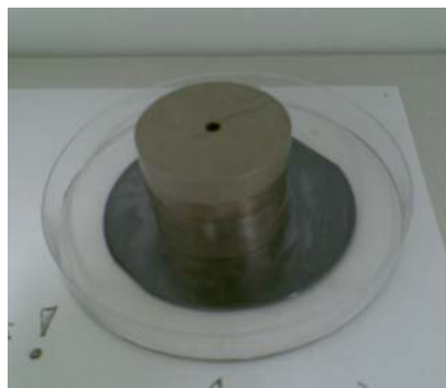
Figure 4.12 PDMS is being cured at room temperature and under pressure.
