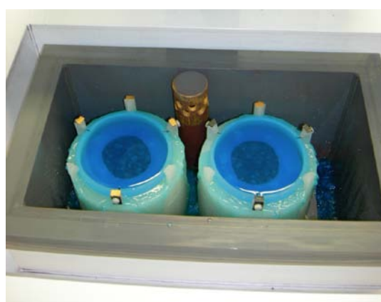
Figure 4.8 Electroplating bath solution is flowing through the Cu pellets (and perforated copper anode) in the bottom of the wafer holder cup.
