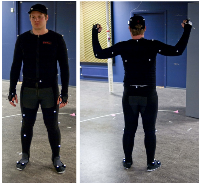
Figure 19. Actor wearing the motion capture suit and markers
