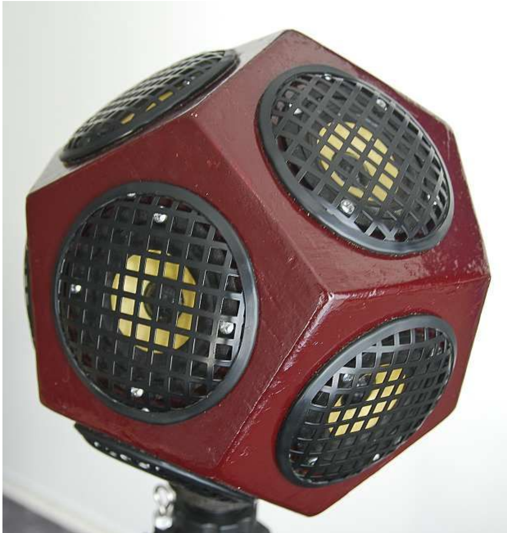
Figure 5: Dodecahedron loudspeaker (adopted from [19])
