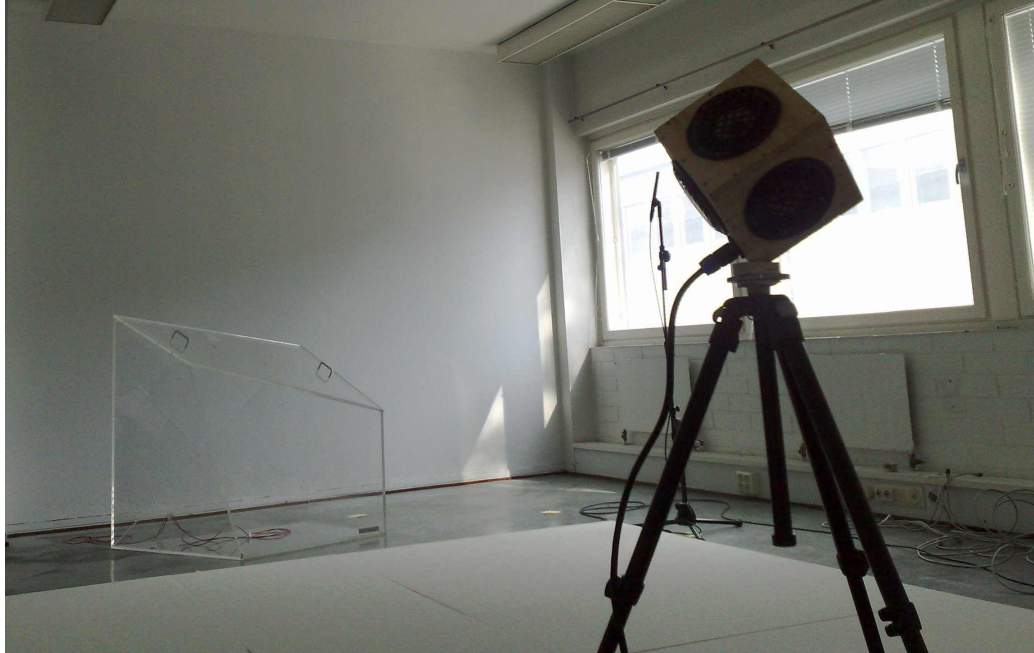
Figure 17: The reverberation room with the sample material installed
