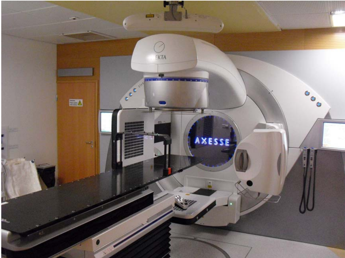
Image 2: Elekta Axesse in HUCH. The gantry is set at a position of 0^\circ . Opposite to the gantry is the flat-image detector for megavoltage radiation. The x-ray tube is on the right in the image and the detector for kilovoltage radiation is opposite to it. In the sealing is an infrared stereo tracking camera and on the treatment table is attached a frame of passive reflectors. On the wall on the very left in the image are the lasers for longitudinal and vertical patient positioning.
