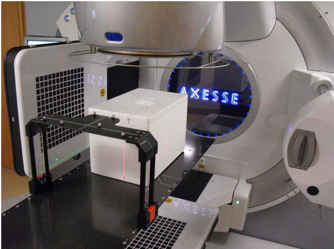
Image 10: The internal organ phantom positioned on the treatment table for CBCT investigations.
