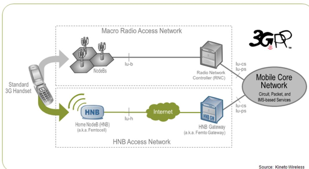
Graph 9: Femtocell Network Architecture - Source: Kineto Wireless.
