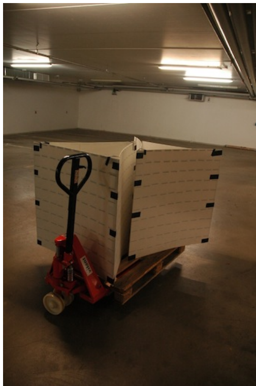
Figure 26: Pallet with 6 sheets of PS plastic holding total of 600 UPM Belt tags.
