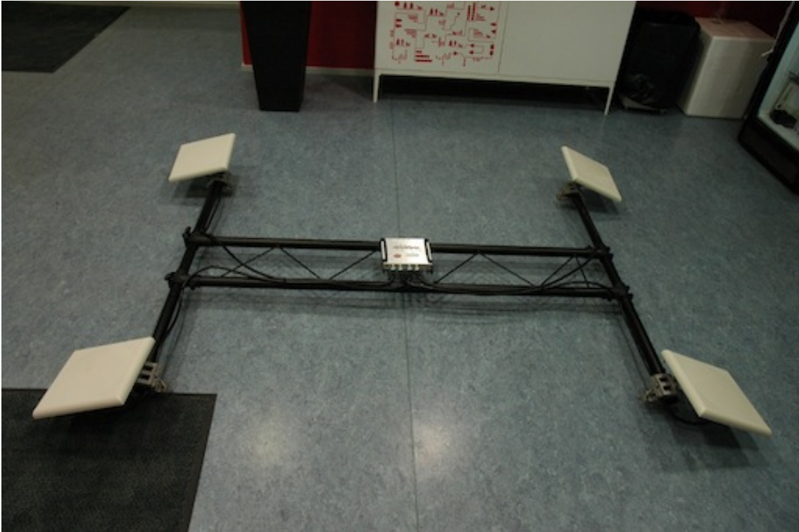
Figure 24: Light roof portal assembly for lay around tag detection using direction sensing methods.
