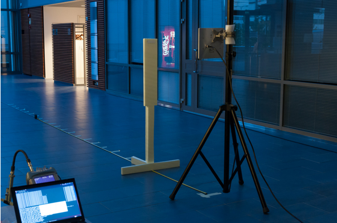
Figure 27: Test setup to measure phase angle rotation and RSSI over distance.
