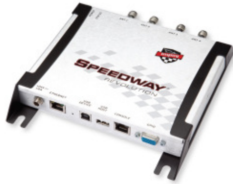
Figure 3: Impinj Speedway Revolution UHF RFID Reader
