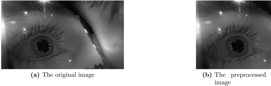
Figure 6.2: Preprocessing the eye image. Figure (a) shows the original image. The image shows parts of the gaze tracking glasses. Figure (b) shows the preprocessed image. Preprocessing reduces the size of an image by selecting only the area of interest. In addition, noise is reduced by Gaussian filtering.
