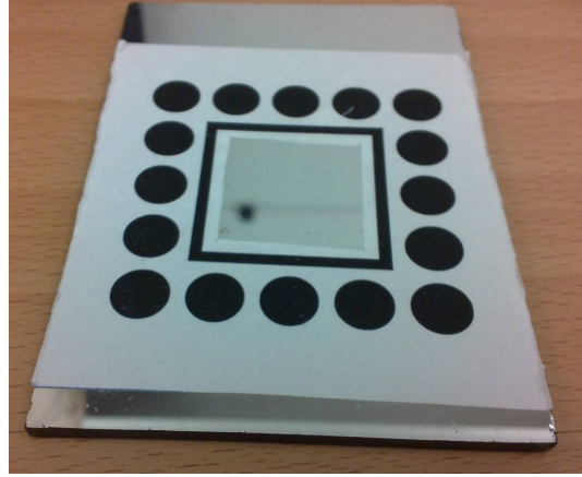
(b) The calibration pattern on a mirror
