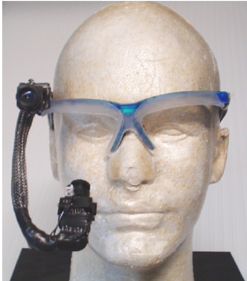
(a) Gaze tracking glasses used in the openEyes project
