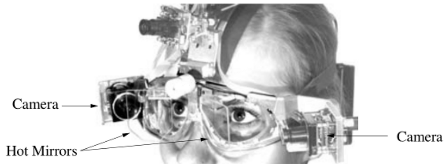
(b) Eye tracking glasses using hot mirrors
