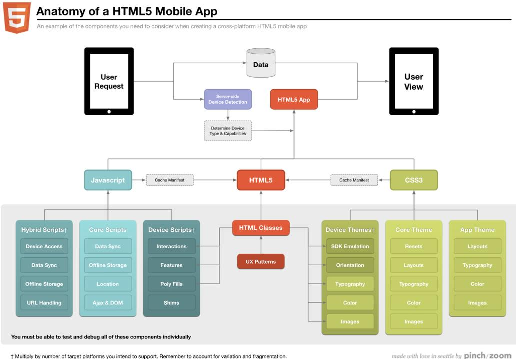
Figure 4.1: HTML5 Mobile Application Anatomy according to [16].
