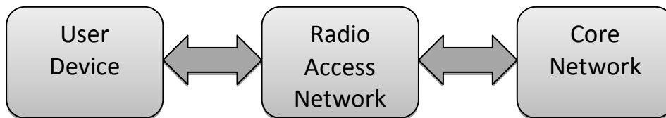
Figure 2. Functional domains of a mobile network
