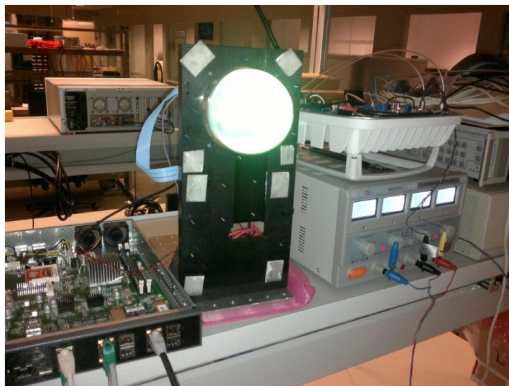
Figure 16: BRAWE receiver employing a lens antenna (in the middle) integrated to a NSN FlexiPacket Radio (right, on top of a regular power source) and to the Lanner MR-730 (left).
