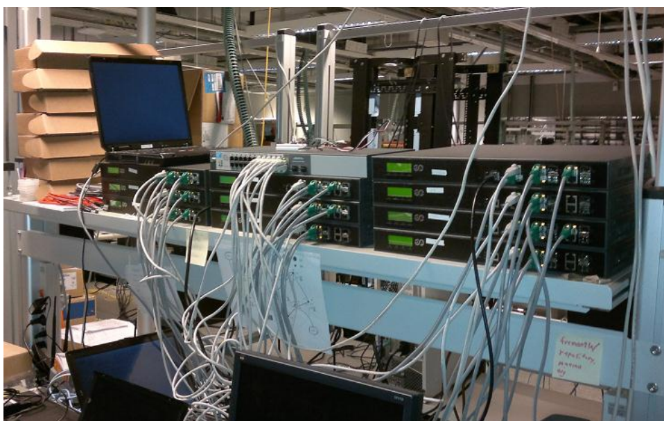
Figure 15: The wireless mesh network demonstrator in the NSN Mobile Backhaul Advanced laboratory. Ten Lanner MR-730 units forming the partial mesh and an Ethernet switch to deliver external synchronization.
