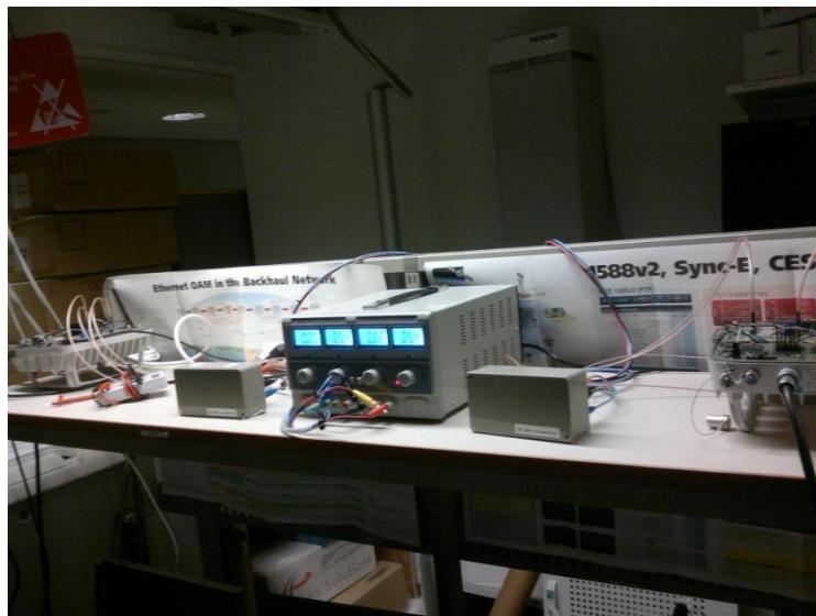
Figure 17: Two transmitter units (grey boxes on both sides of the power source) and NSN FlexiPacket Radios on far right and left side.
