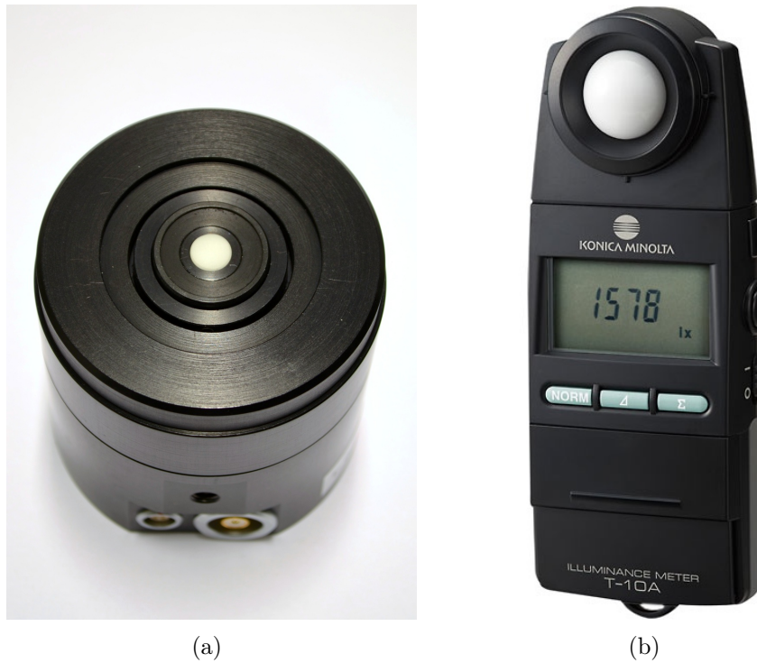
Figure 3: Photograph of (a) PRC Krochmann photometer head with raised diffuser and (b) Konica Minolta T-10A illuminance meter with shaped diffuser [Konica Minolta website].
