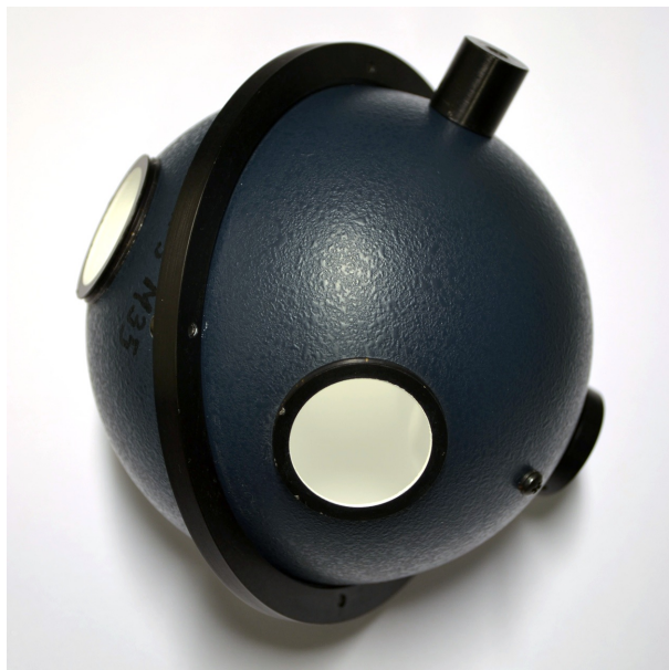
Figure 1: Integrating sphere with two entrance ports open. Global irradiance can be measured by exposing one of the ports to radiation and measuring the light level inside the sphere through the second port. Purpose-built integrating sphere detector heads for spectral irradiance measurements are commercially available.
