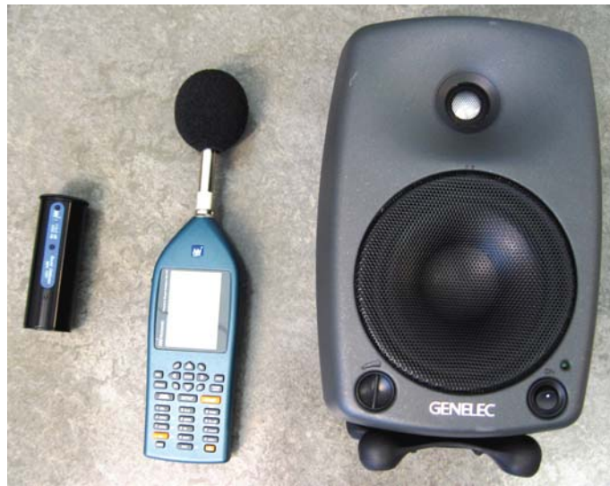
Figure 21: Measurement devices for the healthcare space and for the classroom. From left: class 1 calibrator Norsonic Nor 1251, sound level meter Norsonic Nor140, and loudspeaker Genelec 8030A.
