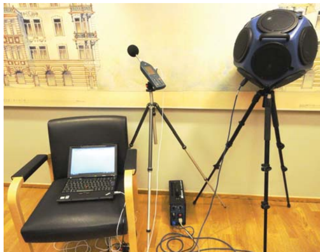
Figure 22: Measurement devices for the open plan office. From left: Lenovo X200 laptop, sound level meter Norsonic Nor140, Norsonic Power Amplifier Nor280, and omnidirectional loudspeaker Norsonic Nor270.
