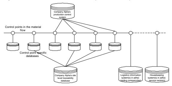
Figure 4: Material flow and the traceability information systems.
