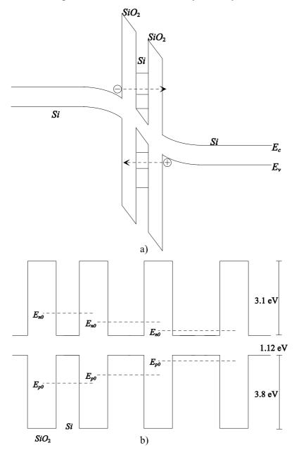
**Figure 1.1** Schematic illustration of energy band structure of a a) RTD b) silicon/silicon dioxide heterostructure.  $E_{p0}$  and  $E_{n0}$  represent the ground state energies in the potential wells.
