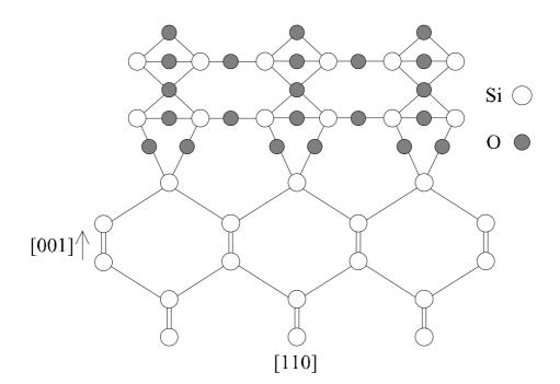
**Figure 2.3** Schematic illustration of silicon/silicon dioxide tridymite structure <sup>43</sup>.
