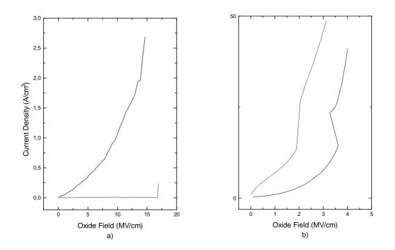
**Figure 5.11** Measured currents through ultrathin silicon dioxide layers ( $d_{ox} \approx 2 - 2.5$  nm).<sup>2</sup>
