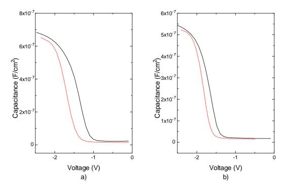
**Figure 5.24** High frequency capacitance from thin oxide MOS samples (dashed red line before and solid black line after annealing). Oxide thickness is a) 4.75 nm and b) 6 nm.
