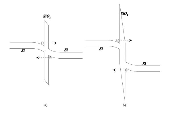
Figure 2.4 Tunneling in an MOS structure: a) direct tunneling b) Fowler-Nordheim tunneling.
