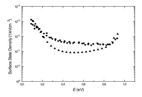
**Figure 5.15** Surface state densities from samples plasma oxidized at room temperature (oxide thickness: down triangles 2 nm, up triangles 3 nm and squares 5 nm).<sup>4</sup>
