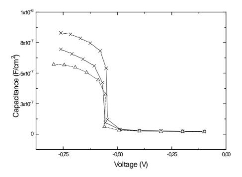
**Figure 5.14** Capacitance as a function of gate voltage from samples plasma oxidized at 700  $^{0}$ C (crosses) and 800  $^{0}$ C (triangles).<sup>4</sup>
