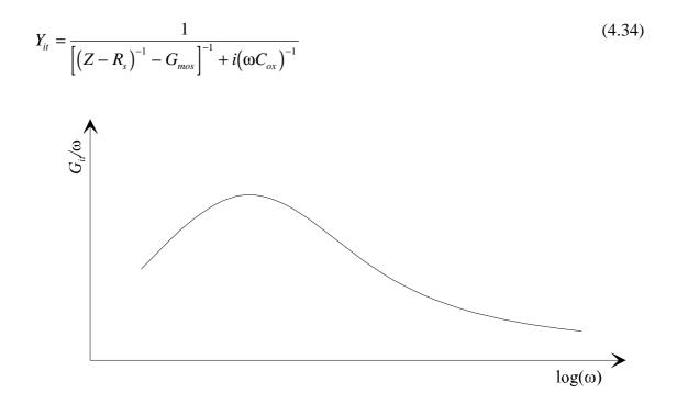
Figure 4.7 A schematic illustration of trap conductance as a function of angular frequency.
