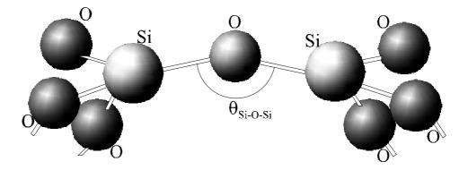
Figure 2.2 Schematic illustration of SiO<sub>4</sub> tetrahedras joined by bridging oxygen.
