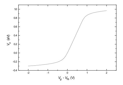
**Figure 4.1** Potential at the oxide/silicon interface of an MOS structure ( $N_A = 10^{16}$  cm<sup>-3</sup>,  $d_{ox} = 2$  nm) as a function of gate voltage.
