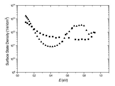
**Figure 5.16** Surface state densities from two MOS samples with about 3 nm silicon dioxide layers, both plasma oxidized in 700  $^{\rm O}$ C.<sup>4</sup>
