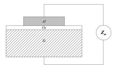
Figure 5.21 Schematic illustration of the MOS structure.
