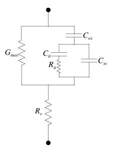
**Figure 4.4** Equivalent circuit of MOS structure.  $G_{mos}$  is the leakage conductance through the structure,  $C_{ox}$  is the metal-oxide-semiconductor capacitance,  $C_{it}$  is the capacitance of the interface traps,  $R_{it}$  is their resistance,  $C_{sc}$  is the depletion region capacitance and  $R_s$  is the series resistance.
