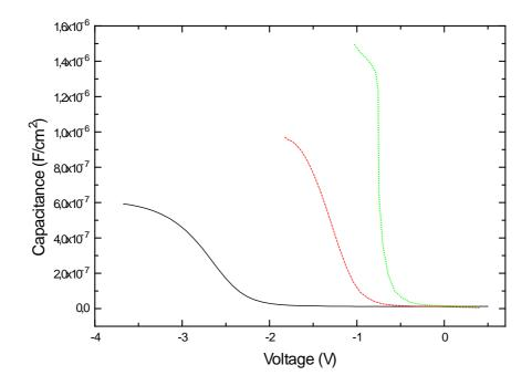
**Figure 5.17** Capacitance as a function of gate voltage from samples plasma oxidized at room temperature. (Oxide thickness: solid black line 5 nm, dashed red line 3 nm and dotted green line 2 nm).  $^4$
