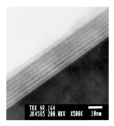
Figure 5.7 TEM picture of a silicon/silicon dioxide heterostructure.
