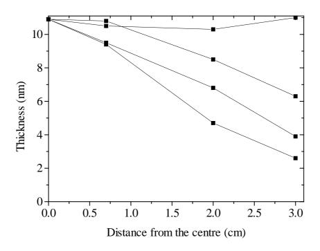
Figure 5.6 Thickness profile of a silicon dioxide layer in four directions from the center. The sample was processed at 800  $^{\circ}$ C for 30 minutes with a corroded heating element.<sup>1</sup>
