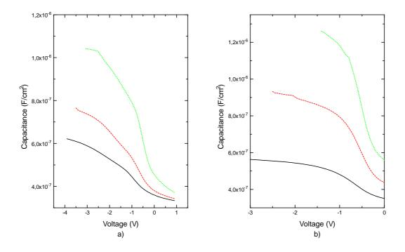
**Figure 5.20** Measured high frequency capacitances after annealing at a) 300  $^{\circ}$ C and b) 750  $^{\circ}$ C  $^{3}$  (oxide film thicknesses from 2.6 to 5.8 nm).
