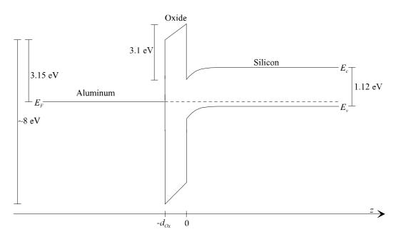
**Figure 2.1** Energy band structure of an aluminum/silicon dioxide/p-type silicon structure with zero bias.
