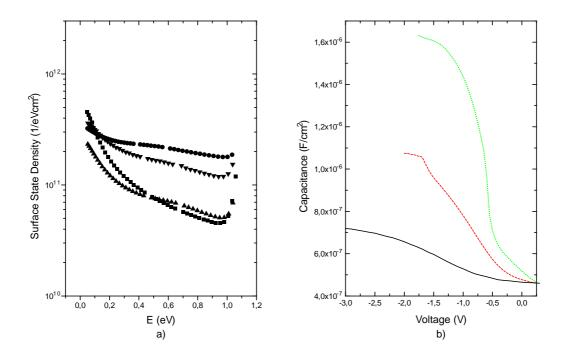
**Figure 5.18** Measured a) surface state densities (squares 2 nm, up triangles 3 nm, down triangles 4.6 nm and circles 5 nm oxide film) and b) high frequency (1 MHz) capacitances (dotted green line 2 nm, dashed red line 3 nm and solid black line 5 nm oxide) from samples fabricated without any post oxidation annealing.<sup>3</sup>
