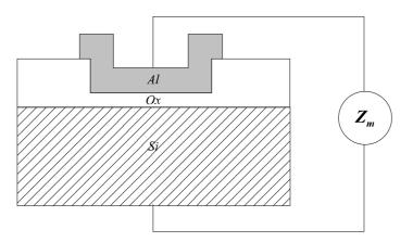
Figure 5.8 Schematic illustration of the MOS structure.
