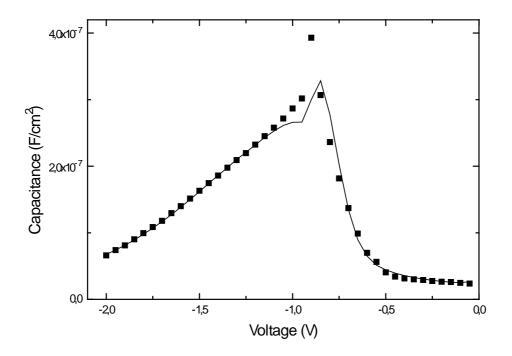
**Figure 4.5** Measured (squares) and calculated (solid line) capacitance of the same MOS structure as in Figure 4.3. The calculation is based on the following parameters: Oxide thickness 3.9 nm, series resistance 310  $\Omega$ , doping density 4.10<sup>15</sup> 1/cm<sup>3</sup>, and flat band voltage -0.68 V.
