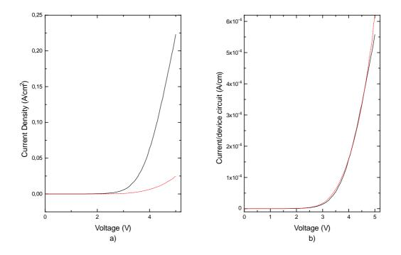
**Figure 2.6** Measured a) average current density b) current divided by the length of device periphery, through two MOS structures. (Solid black line: Device area  $(100 \,\mu\text{m})^2$ . Dashed red line: Device area  $(1 \,\text{mm})^2$ .)
