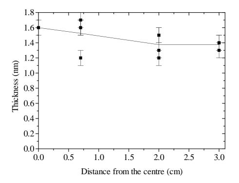
**Figure 5.5** Thickness profile of a silicon dioxide layer processed at 750  $^{\circ}$ C for 30 minutes. The solid line is averaged from the measured values from four directions from the center. The measurements are presented as squares.<sup>1</sup>
