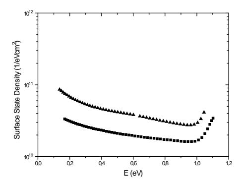
**Figure 5.19** Measured surface state density after annealing at 750  $^{\rm O}$ C (triangles) and 300  $^{\rm O}$ C (squares). Film thickness around 4 nm. <sup>3</sup>
