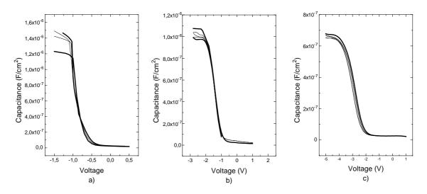
**Figure 5.9** Measured capacitance of MOS samples fabricated with a) two, b) three and c) five oxidation cycles (frequency 1 MHz). Thick lines represent the calculated error limits.  $^2$
