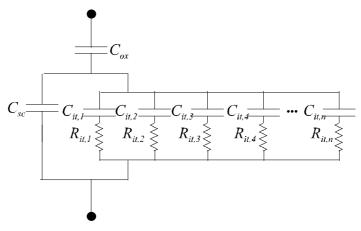
Figure 4.6 Equivalent circuit of the MOS capacitor in depletion for a distribution of single-level interface traps (leakage  $G_{mos}$  excluded).
