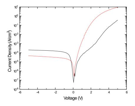
**Figure 2.5** Measured average current density through MOS structures with ultrathin silicon dioxide layer; device area  $(100 \,\mu\text{m})^2$  solid black line,  $(500 \,\mu\text{m})^2$  dashed red line.
