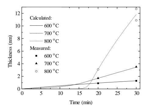
**Figure 5.3** Measured thickness of the silicon dioxide layer as a function of time at various temperatures  $^{1}$ . The calculations are based on equations (5.3) and (5.4) which are fitted with the measurements.
