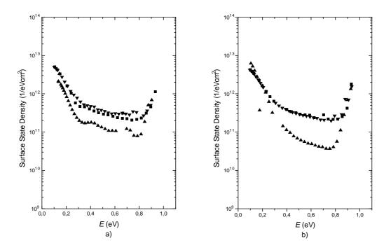
**Figure 5.13** Surface state densities from samples plasma oxidized at a) 700  $^{\circ}$ C (oxide thickness: up triangles 2.5 nm, squares 3 nm and down triangles 3.4 nm) and b) 800  $^{\circ}$ C (oxide thickness: up triangles 2 nm, squares 4.2 nm and down triangles 4.4 nm). <sup>4</sup>
