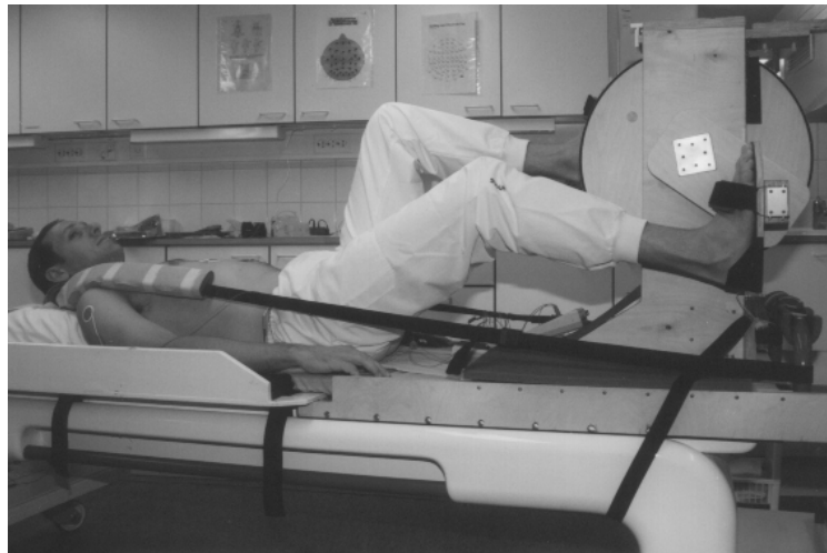
Fig. 3: The non-magnetic exercise ergometer used in the MCG and the BSPM measurements.
