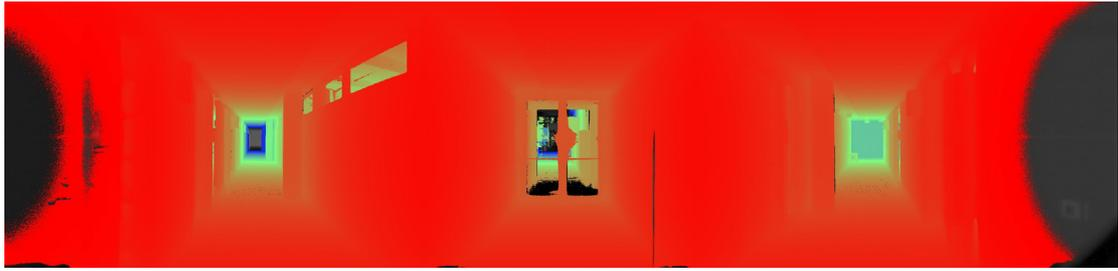
Figure A.15 An illustration of the range image "scan5". Ranges between 1.0 and 20.0 meters have been pseudo-colored from red to blue, respectively.
