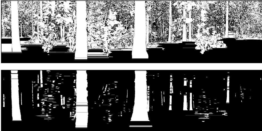
Figure B.5 Initial segmentation of the range profile data "scanR" in the upper image. In the lower image, the valid circle models, computed from the segments in the upper image, are shown.
