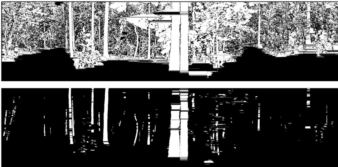
Figure B.6 Initial segmentation of the range profile data "scanQ" in the upper image. In the lower image, the valid circle models, computed from the segments in the upper image, are shown.
