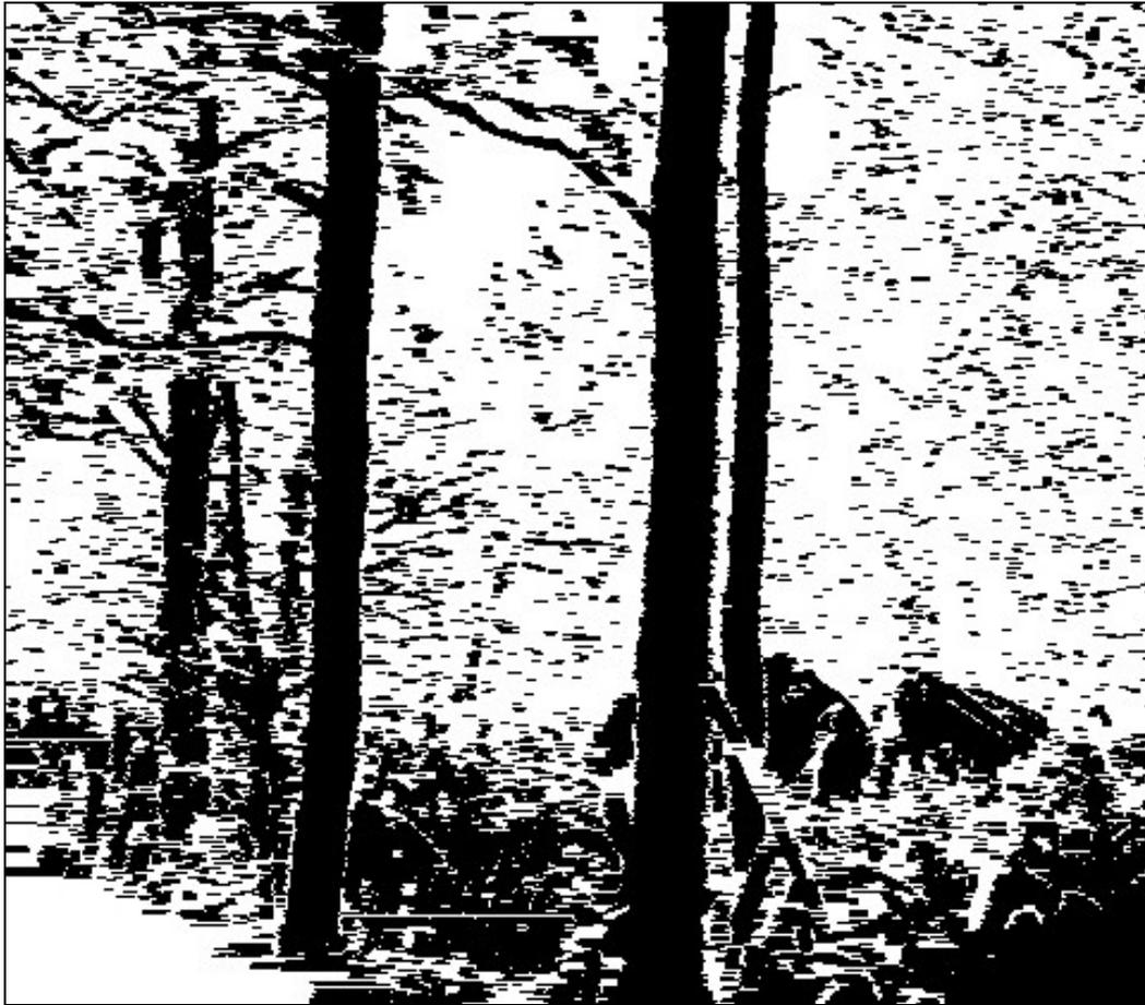
**Figure 4.9** Horizontal segments extracted from the range image, presented in Figure 4.8. The range segments, the length of which was found to be between 0.06 and 1.0 meters, have been painted black.
