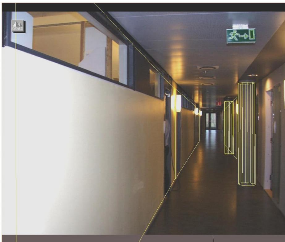
**Figure 6.6** A partial, mixed reality view of a 3D feature model. The wall plane objects and the cylinder models for the pillars have been extracted from the range image labeled "scan1". The complete set of feature objects extracted from the range image can be seen in Figure D.19.
