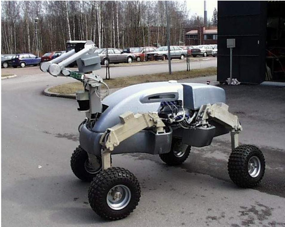
**Figure 2.6** WorkPartner, the prototype of a mobile service robot designed to work interactively with humans in outdoor environments. The robot is equipped with a 2D laser scanner used for autonomous, model-based navigation.
