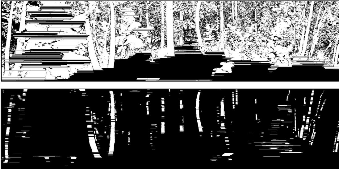
Figure B.3 Initial segmentation of the range profile data "scanT" in the upper image. In the lower image, the valid circle models, computed from the segments in the upper image, are shown.
