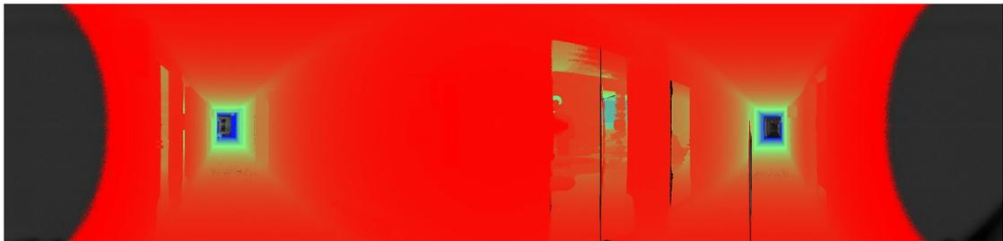
Figure A.17 An illustration of the range image "scan7". Ranges between 1.0 and 20.0 meters have been pseudo-colored from red to blue, respectively.
