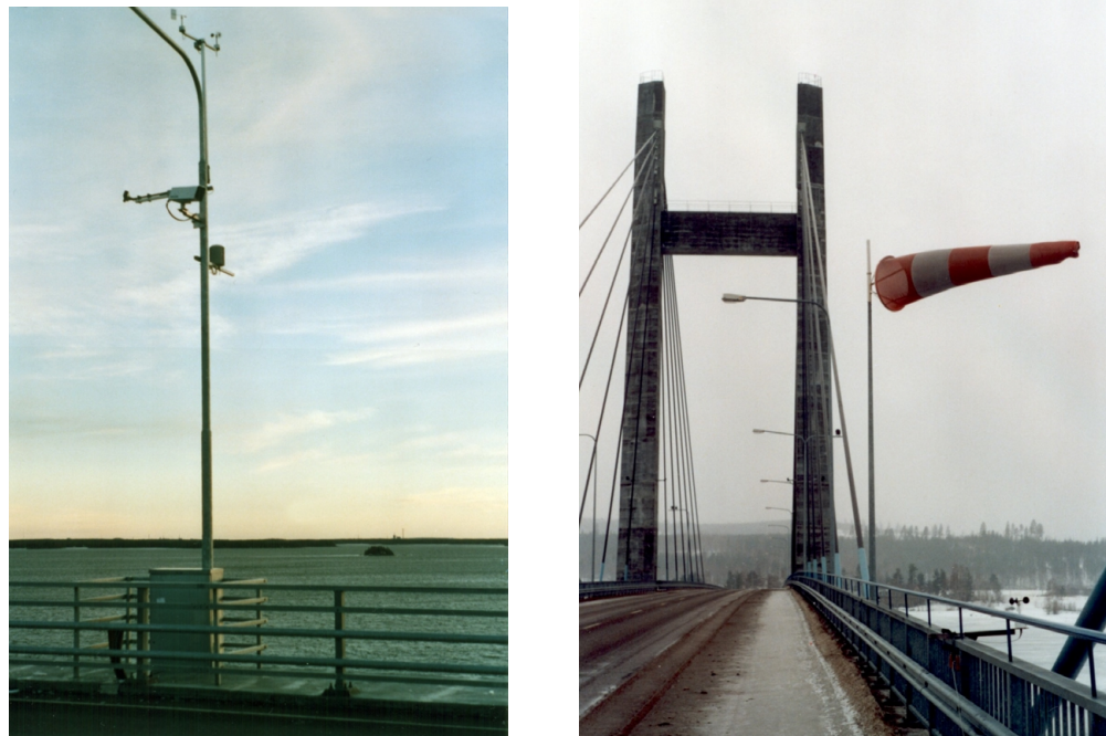
Fig. 24 Left: the road weather station of the Raippaluoto Bridge with wind velocity and direction measurement capabilities. Right: the analog wind vane of the Kärkinen Bridge and the cup anemometer's positioning to the railing. Photos by the author.
