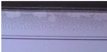
Figure 4.2 Starting of delamination on the side edge of the back contact on 1 x 1 ft 2 a-Si module AB507 after 50 cycles of thermal cycling test.
