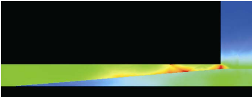
Figure 5.18. Amplitude distribution of the electrical field in a sapphire wedge. Vertical ( E ) plane, frequency 75 GHz.
