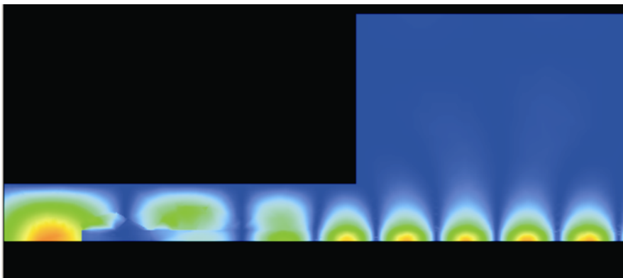
Figure 5.16. Electrical field in a sapphire wedge at a particular time instance at 75 GHz. Horizontal ( \mathbf{H} ).
