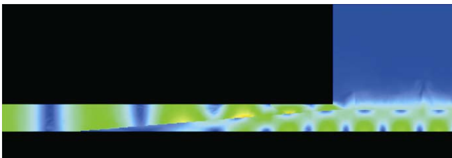
Figure 5.20. Electrical field distribution in a sapphire wedge at a particular time instance. Vertical ( E ) plane, frequency 90 GHz.
