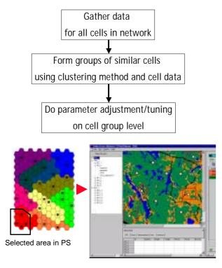
Figure 2. Example of utilisation of cluster information in optimisation process. Selection for cells to be optimised/autotuned. PS stands for performance spectrum.
