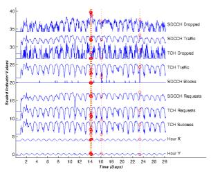
Figure 4 Scaled performance indicators analysed using moving 14-day profile training. The anomalies are marked with red dotted vertical lines. The first 14 days were only used for profile training and therefore not analysed.
