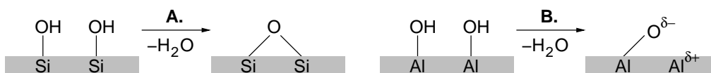
Figure 2.2: Schematic presentation of dehydroxylation: (A) the formation of siloxane bridges on silica and (B) the formation of c.u.s. Al–O pairs on alumina.
