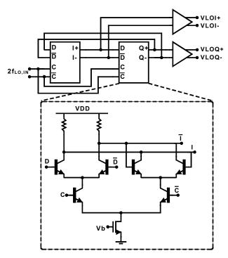
Fig. 4. Schematic of the LO divider.
