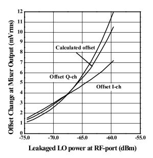
Fig. 3. Measured and calculated DC-offset change, when RF voltage gain is changed 20 dB.
