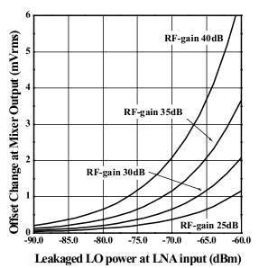
Fig. 2. Calculated DC-offset change at mixer output as a function of LO power leakage to LNA input, when the RF front-end gain is lowered by 3 dB.
