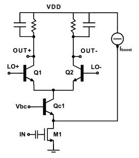
Fig. 5. Schematic of the used mixer.
