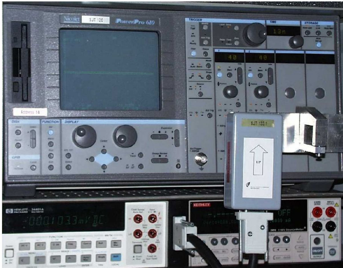
Figure 9 Typical setup of the calibration system. The device under calibration is a digitizer (top). The calibrator head is connected directly to its input. A multiwire cable connects the head to an adapter box (not shown). The adapter is connected to the rear terminals of the direct voltage source (bottom right) and multimeter (bottom left). The controlling computer is not shown.
