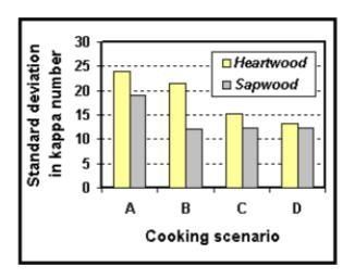
*Fig. 9*. *Standard deviation in kappa number within the handmade chips.* (Calculated from all FTIR data)
