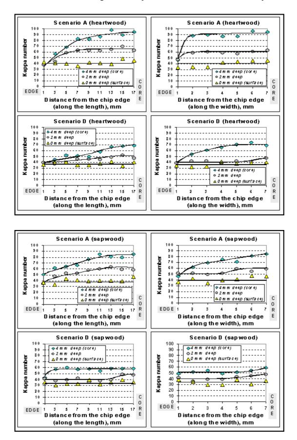
**APPENDIX I.** Delignification profiles within the handmade chips.
