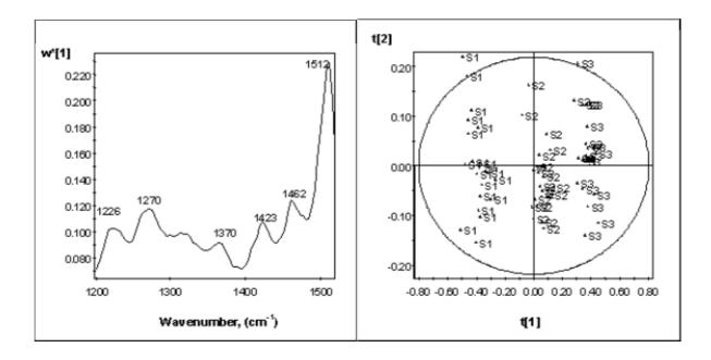
*Fig. 3. PLS loading spectrum of the first component and PLS*  $t_1/t_2$  *score plot of the calibration data set.*
