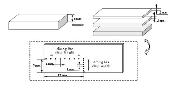
Fig. 2. Preparation of test-pieces and selection of the points for FTIR analysis.
