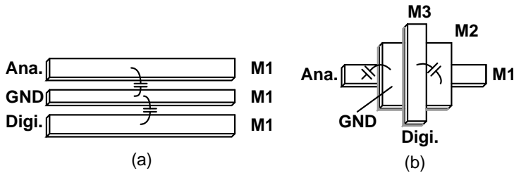
Figure 5.3 Isolation of (a) parallel and (b) crossing analog (Ana.) and digital (Digi.) signals using ground plate (GND) in between.
