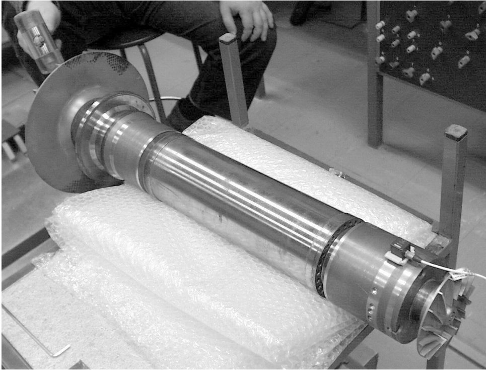
Fig. 3.3 Measurement of the bending critical speeds of the laminated rotor. On the right, an acceleration sensor is attached. The rotor lies on an air bubble matrix.
