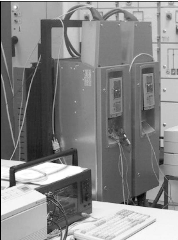
Fig. 6.1 A photograph and data of the frequency converters used to supply the 60 kW 60000 1/\text{min} high-speed machines in the back-to-back test setup. Converters in the picture are fitted side by side in the rack, power cables above connecting the DC-links.
