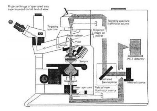
Figure 7. Cross-sectional view of an FT-IR microscope (Wilson 1995).
