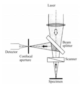
Figure 6. Diagrammatic presentation of an incident light confocal system shows the excitation beam and the reflected fluorescent light (Brooker 1995).
