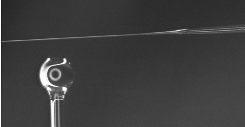
Figure 10: Etch-eroded fiber coupler (horizontal structure), with silica microsphere. Sphere diameter roughly 0.3 mm.
