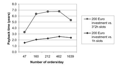
**Figure 5.** Payback time for the investment in delivery box solution compared to the solution with attended reception
