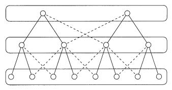
Fig. 2. The structure of a three-level one-dimensional TS-SOM. The solid lines represent parent-child relations and the dash lines represent neighbouring nodes included in the BMU search space.
