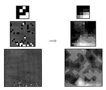
Fig. 6. An example showing how the levels of a TS-SOM, on which the images selected and rejected by the user are shown with white and black marks, respectively, are convolved with low-pass filters.
