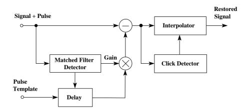
Figure 3.2: Processing stages of the template-matching method for de-thumping. Adapted from [75].
