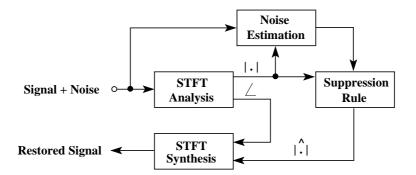
Figure 3.4: STSA-based hiss reduction system. Adapted from [119].
