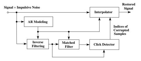
Figure 3.3: Model-based de-clicking method. Adapted from [75].
