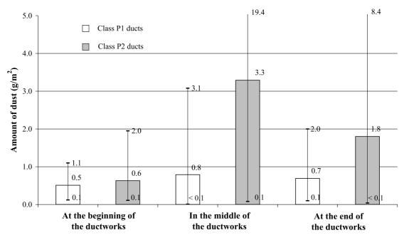
Fig. 1 The mean amount of dust and the range in cleanliness categroy p1 and p2 ductworks
