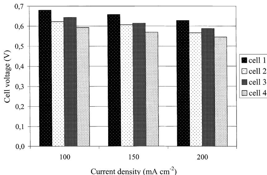
Fig. 7. Individual cell voltages during the measurement of ohmic losses. Air supply: free convection.
