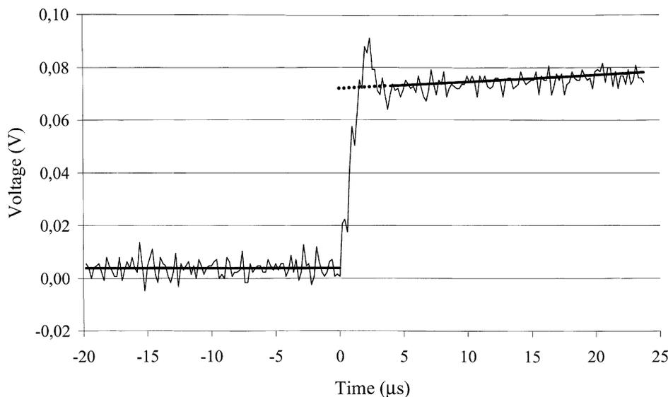
Fig. 2. Voltage transient (thin line) and fitted average voltage (bold line) for the whole stack. Extrapolation is indicated with a dotted line. Air supply: free convection;  $j = 100 \text{ mA cm}^{-2}$ .
