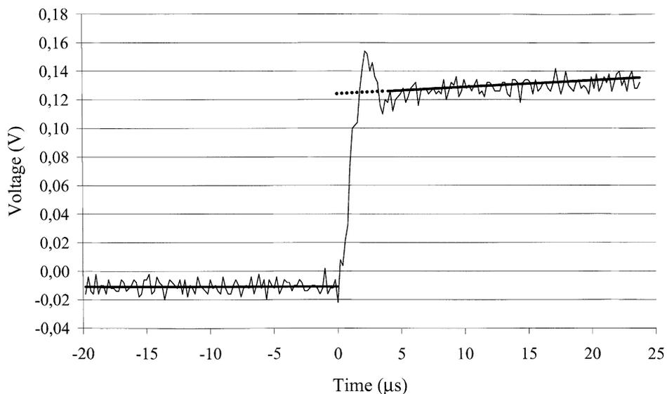
Fig. 4. Voltage transient (thin line) and fitted average voltage (bold line) for the whole stack. Extrapolation is indicated with a dotted line. Air supply: free convection;  $j = 200 \text{ mA cm}^{-2}$ .
