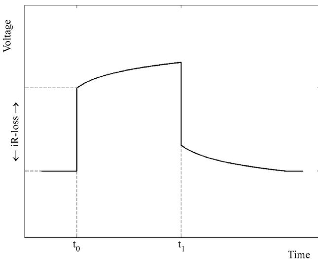
Fig. 1. An ideal voltage transient in a fuel cell after a current interruption. The cell is operated at a fixed current. At  $t = t_0$ , the current is interrupted and the ohmic losses vanish almost immediately. After the current interruption, electrochemical overpotentials start to decay and the voltage rises exponentially towards the open-circuit voltage. At  $t = t_1$ , the current is again switched on.
