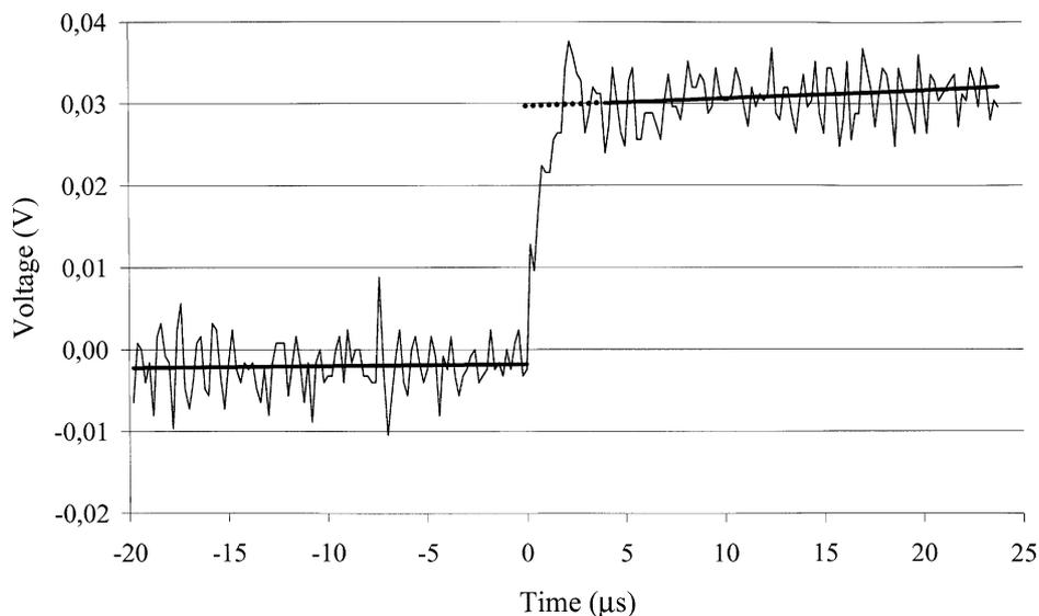
Fig. 9. Voltage transient (thin line) and fitted average voltage (bold line) for an individual cell. Extrapolation is indicated with a dotted line. Air supply: forced convection;  $j = 100 \text{ mA cm}^{-2}$ .
