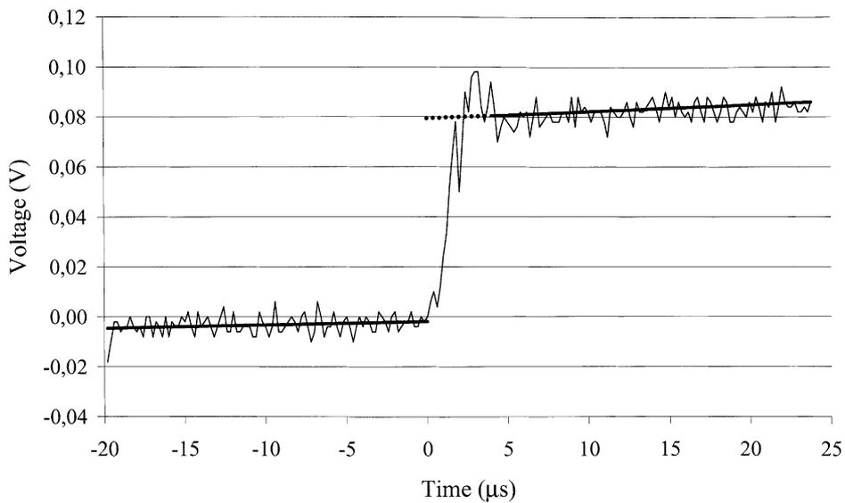
Fig. 11. Voltage transient (thin line) and fitted average voltage (bold line) for an individual cell. Extrapolation is indicated with a dotted line. Air supply: forced convection;  $j = 400 \text{ mA cm}^{-2}$ .
