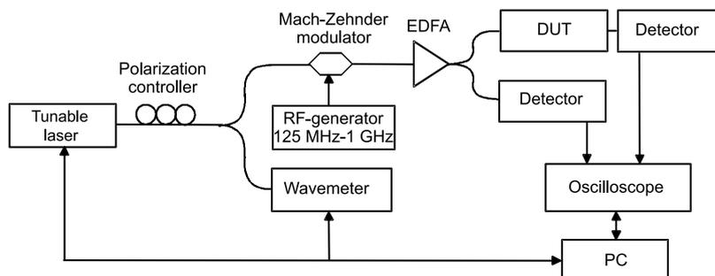
Fig. 1. Experimental setup for group delay measurements using the phase-shift technique.
