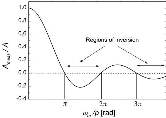
Fig. 2. Normalized amplitude of the measured ripple as a function of  $\omega_m/p$ .
