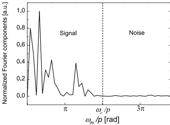
Fig. 5. Fourier spectrum of the measured group delay at 1 GHz versus  $\omega_m/p$ . The vertical dashed line represents the cut-off frequency of the filter applied. The cut-off frequency of the numerical filter was chosen so that  $\omega_c/p = 2\pi$ .
