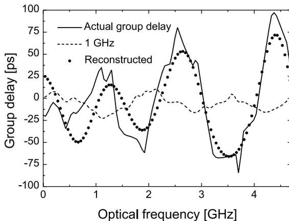
Fig. 6. Reconstruction of the actual group delay of a fiber Bragg grating using the data measured at 1 GHz. The measured data and the actual profile are also plotted.
