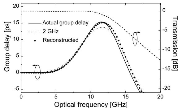
Fig. 7. Reconstruction of the group delay of a narrow-band thin-film filter. The transmission spectrum of the filter is plotted as a dashed line.
