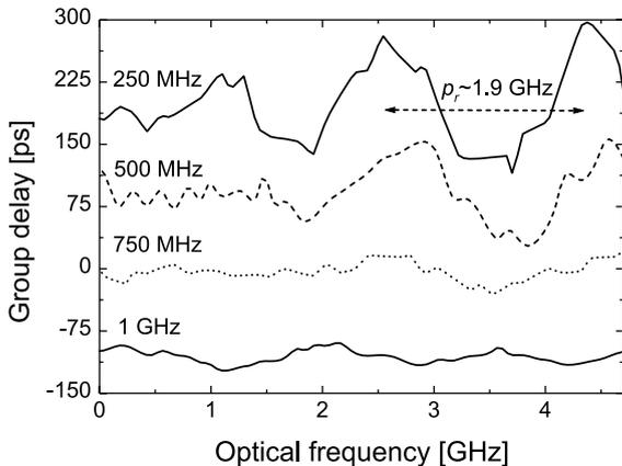
Fig. 3. Traces of the group delay ripple of a fiber Bragg grating for four different modulation frequencies.
