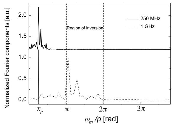
Fig. 4. Fourier spectrum of the measured group delay at 250 MHz versus  $\omega_m/p$  for two different values of  $\omega_m$ . The area delimited by the vertical dashed lines represents the region of inversion and attenuation.
