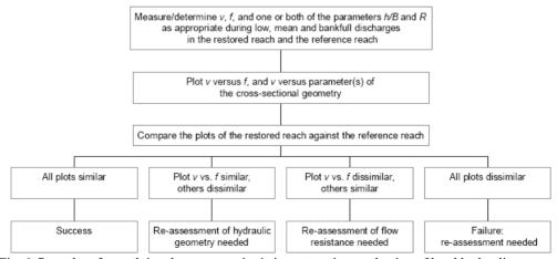
Fig. 6. Procedure for applying the success criteria in post-project evaluation of local hydraulics.
