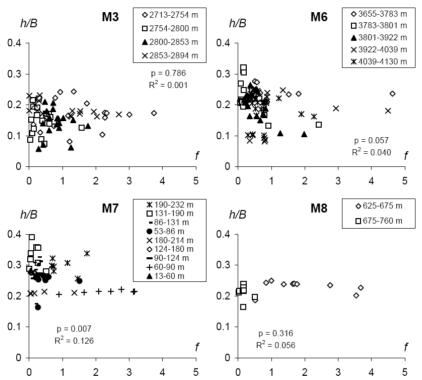
Fig. 4. Depth-width ratio vs. friction factor for sub-reaches of M3, M6, M7 and M8. See text for the statistical parameters R<sup>2</sup> and p.
