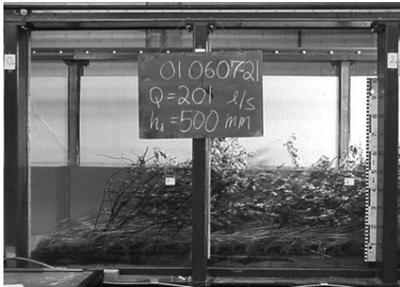
Fig. 3. Test run 010607-21 of series S3_Pa with willows and sedges. The average flow velocity is 38.7 cm/s.
