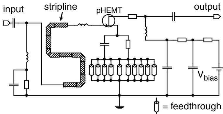
FIG. 6: Amplifier block used in the balanced amplifier configuration of Fig. 5.
