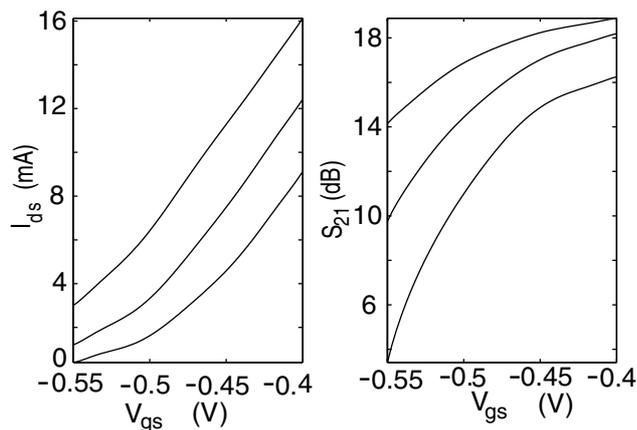
FIG. 2: Drain-source current  $I_{ds}$  (a) and gain  $S_{21}$  (b) as a function of gate voltage. Three different curves correspond to the drain-source voltages of 0.5, 1 and 1.5 V from bottom to the top, respectively.
