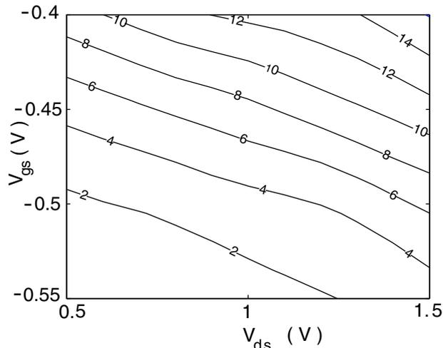
FIG. 1: Constant drain-source current  $I_{ds}$  contours of the pHEMT at 4.2 K in units of mA as a function of bias voltages.
