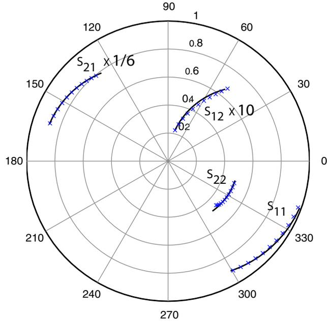
FIG. 4: Comparison between measured pHEMT S-parameters ( $\times$ ) at temperature of 4.2 K and the fitted small-signal model response (line) in polar coordinates.  $S_{21}$  is multiplied by factor 1/6 and  $S_{12}$  by factor 10 in the figure. Frequency range is 500 – 1600 MHz.
