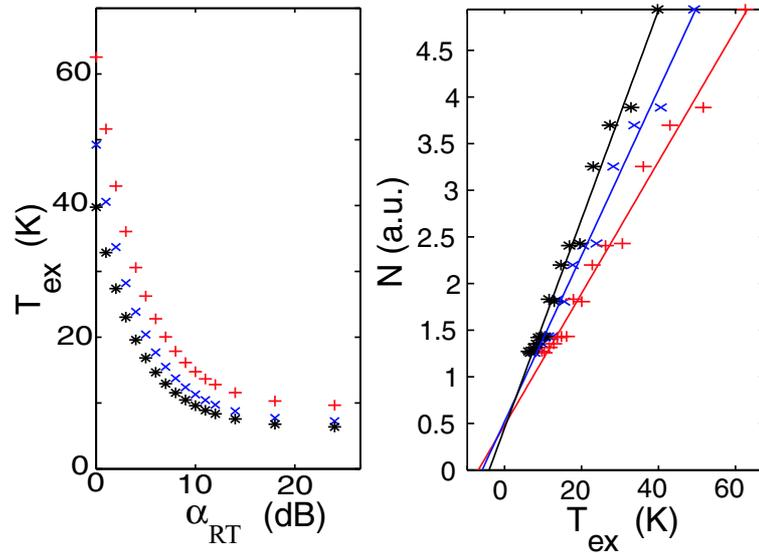
FIG. 10: a) Excess noise  $T_{ex}$  at the amplifier input as a function of the room-temperature attenuation  $\alpha_{RT}$ . b) Typical measured noise  $N$  and a linear fit to extract noise temperature  $T_N$ . Symbols denote the expected value ( $\times$ ) and component values giving minimum (+) and maximum ( $\star$ ) amplifier noise temperature  $T_N$ .
