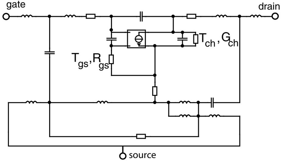
FIG. 3: Small signal model for pHEMT including package parasitics. Network topology is the same as in the data sheet of the manufacturer [10].  $T_{gs}$  and  $T_{ch}$  denote the gate and channel temperatures that are used in the noise model.
