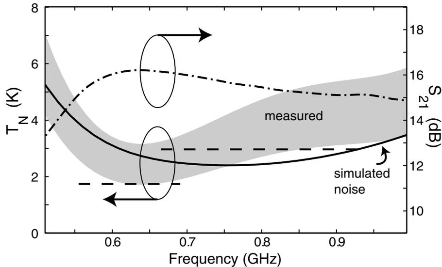
FIG. 11: Measured noise temperature  $T_N$  with error estimate (gray area) and the result from the simulation (solid line). The dashed lines denote reference noise temperatures of two amplifiers taken from Ref. [6]. Amplifier gain  $S_{21}$  is denoted by a dash-dotted line.
