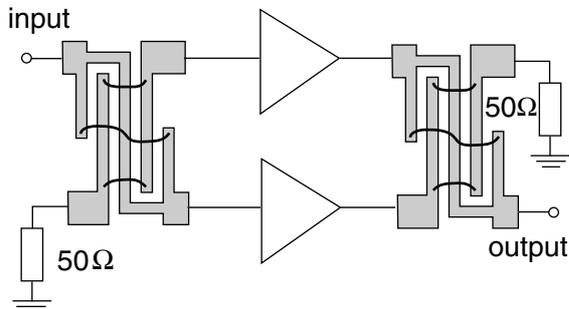
FIG. 5: Schema of the balanced amplifier configuration consisting of two Lange couplers, two  $50 \Omega$  terminations and two amplifier blocks that are illustrated in more detail in Fig. 6.
