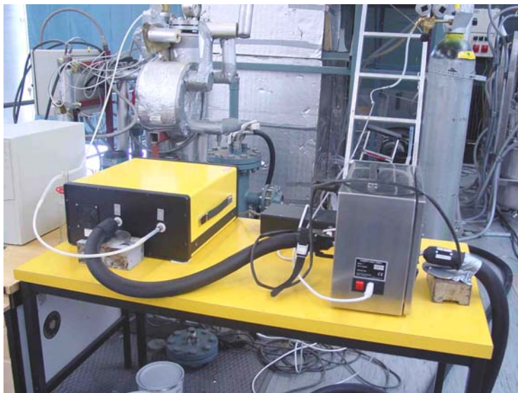
Fig. 4.7 Front view of the DX 4000 FT-IR spectrometer with the sampling system
