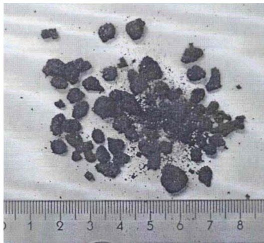
Fig. 5.28 Image of char particles taken from BFB for 100% PVC in two-stage combustion test (scale in centimeters)
