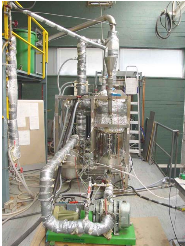
Fig.4.2 Front view of the two-stage combustion test facility (May 2002)
