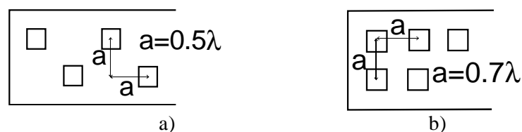
Figure 16. a) Zigzag antenna array used indoors. b) Linear antenna array used outdoors.
