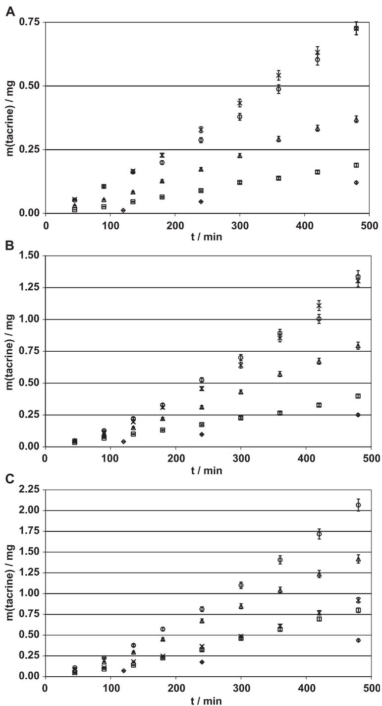
Fig. 2. (a–c) The experimental curves for tacrine release with constant salt concentration, but at different current densities, (a) [NaCl] = 0.15 M, (b) [NaCl] = 0.3 M and (c) [NaCl] = 0.5 M.  $\diamond$ ,  $\square$ ,  $\Delta$ ,  $\times$  and  $\circ$  denote passive diffusion, 0.05, 0.10, 0.25 and 0.50 mA/cm<sup>2</sup> respectively.
