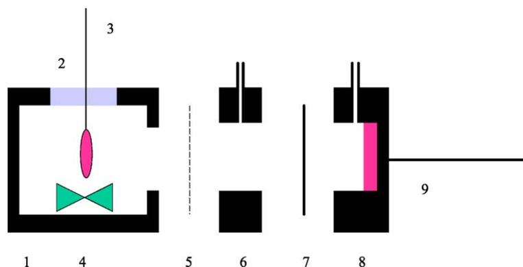
Fig. 1. In vitro iontophoretic cell. (1) The return compartment, (2) lid, (3) Ag/AgCl electrode, (4) magnetic stirrer, (5) porous membrane, (6) donor compartment including the ion-exchange material, (7) Nafion<sup>®</sup> membrane, (8) electrode compartment, (9) Ag/AgCl electrode.
