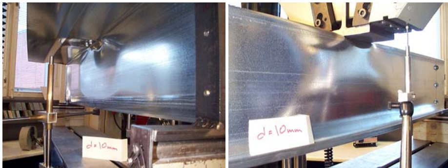
Fig. 3.43 Deformations in specimen IOF200-t15-S1000-2 at time when top flange displacement is equal to 10 mm, views from left and right side.
