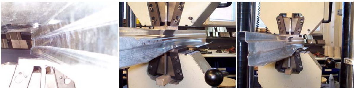
Fig. 3.9 Web crippling progression in test ITF100R-t10-1.
