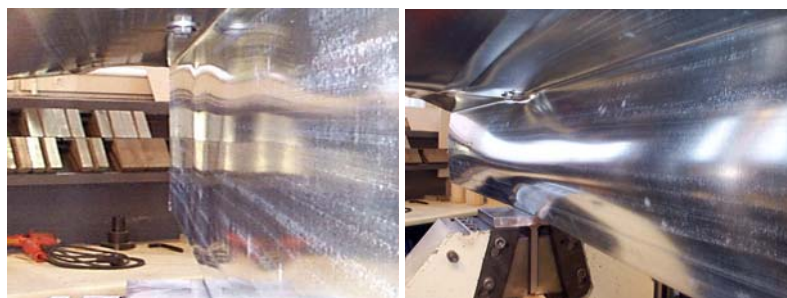
Fig. 3.19 Web crippling progression in test ITF200-t10-2.
