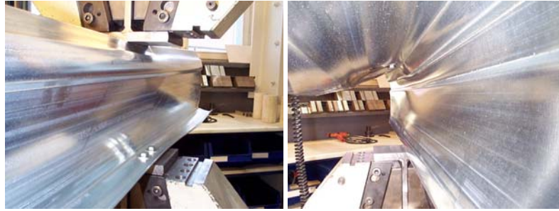
Fig. 3.20 Web crippling progression in test ITF200R-t10-1.
