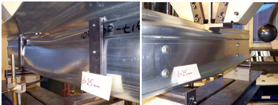
Fig. 3.38 Deformations in specimen IOF200R-t15-S600-1 at time when top flange displacement is equal to 25 mm, views from left and right side.
