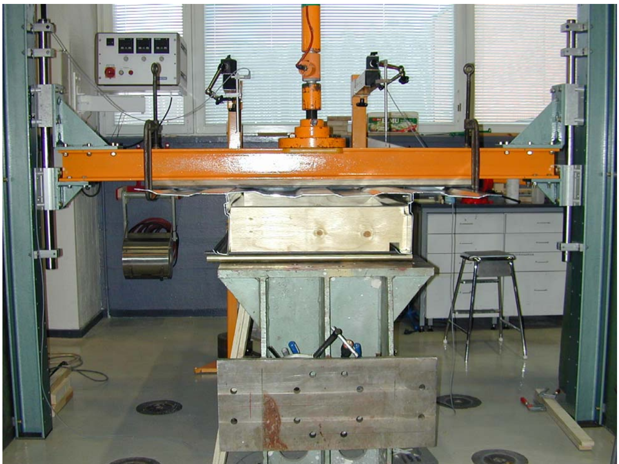
Fig. 3.52 General view of test set-up for S-IOF-tests on built-up specimens.
