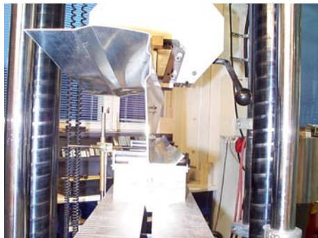
Fig. 3.39 Deformations in specimen IOF200R-t15-S600-1 at time when top flange displacement is equal to 20 mm, axial view from end of beam.
