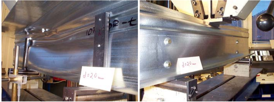
Fig. 3.37 Deformations in specimen IOF200R-t15-S600-1 at time when top flange displacement is equal to 20 mm, views from left and right side.
