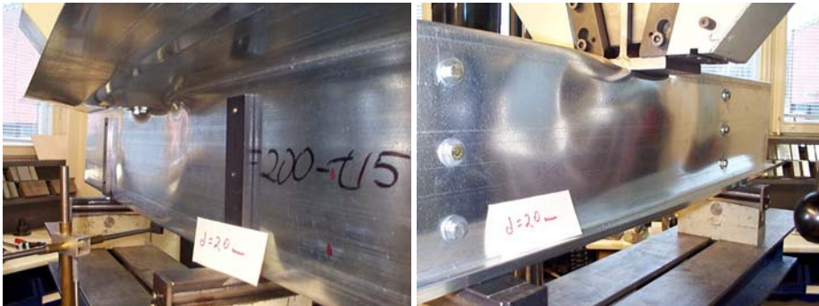
Fig. 3.31 Deformations in specimen IOF200-t15-S600-1 at time when top flange displacement is equal to 20 mm, views from left and right side.
