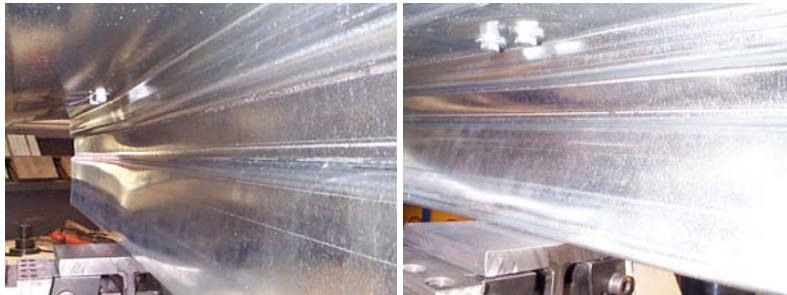
Fig. 3.16 Web crippling progression in test ITF150R-t15-1 as seen from the "underside".
