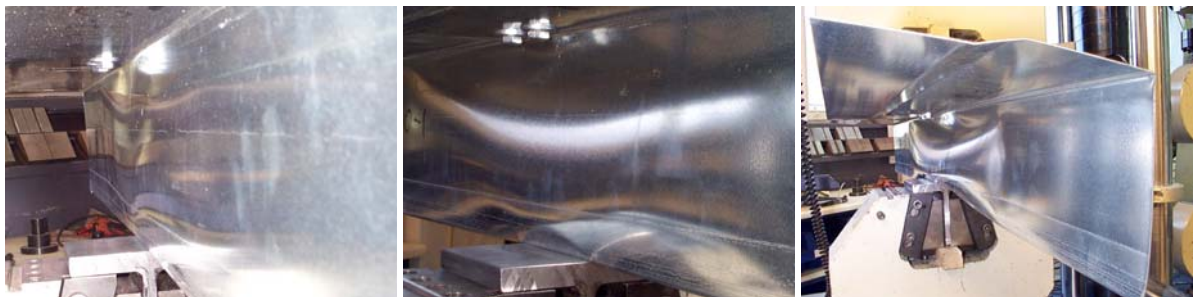
Fig. 3.11b Web crippling progression in test ITF150-t10-1 as seen from the "underside".
