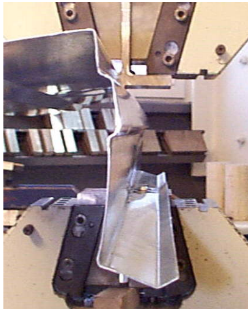
Fig. 3.13 Web deformation in test ITF150R-t10-2.
