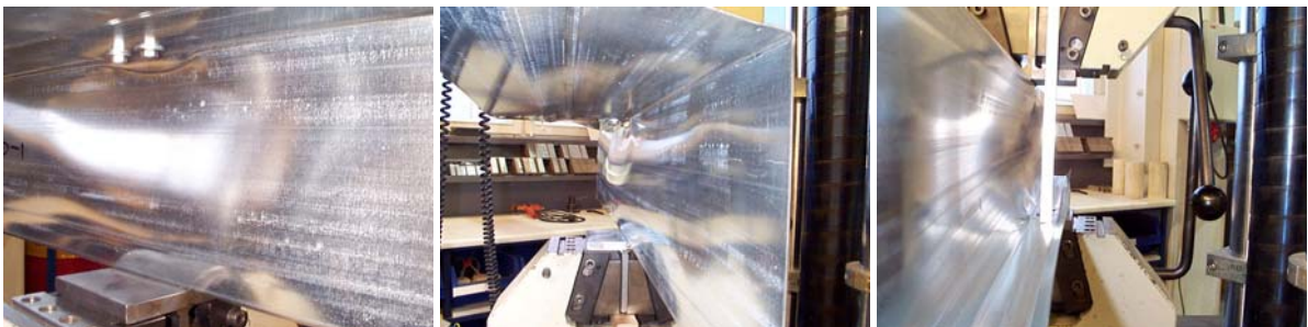
Fig. 3.18 Web crippling progression in test ITF200-t10-1.
