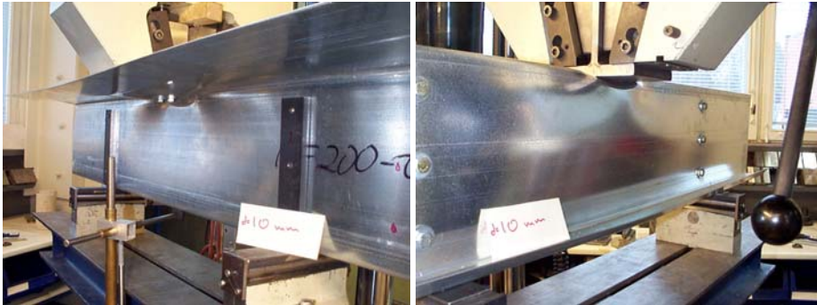
Fig. 3.30 Deformations in specimen IOF200-t15-S600-1 at time when top flange displacement is equal to 10 mm, views from left and right side.
