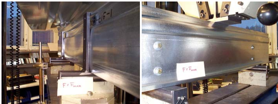
Fig. 3.35 Deformations in specimen IOF200R-t15-S600-1 at load F = F_u , views from left and right side.
