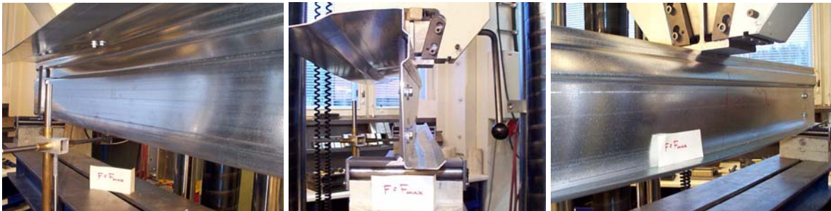
Fig. 3.48 Deformations in specimen IOF200R-t15-S1000-1 at load F = F_u , views from left side, beam end and right side.
