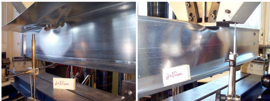
Fig. 3.44 Deformations in specimen IOF200-t15-S1000-2 at time when top flange displacement is equal to 20 mm, views from left and right side.
