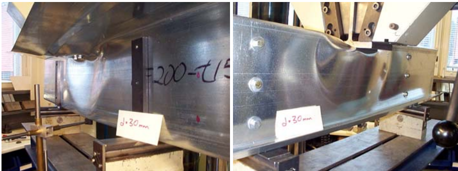
Fig. 3.32 Deformations in specimen IOF200-t15-S600-1 at time when top flange displacement is equal to 30 mm, views from left and right side.
