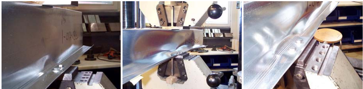
Fig. 3.11a Web crippling progression in test ITF150-t10-1 as seen from the "outside".
