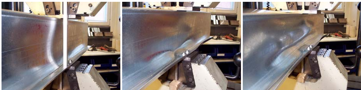
Fig. 3.23 Web crippling progression in test ITF200-t15-1.
